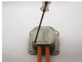
Abschirmdeckel festschrauben Tighten rear screen plate
